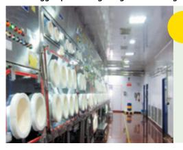
At our API Chennai facility, we have installed a containment (Isolator ) facility to handle the cytotoxic drugs. Isolators are the key control measure in preventing employee exposure to cytotoxic drugs, many of which are classified as hazardous to health. The facility also protects the product from microbiological contamination during production. Negative pressure isolators are designed to give optimal protection to the operator.
